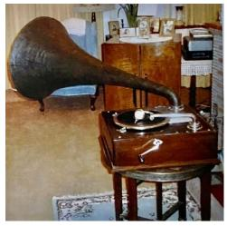
may be interesting to remember that the 'Exhibition' box was used on all G&T/HMV gramophones from 1904 to 1924, and modified versions were used on EMG gramophones, including mine, for a few years after that.) The clockwork motor is a single-spring COLLARO Model M2. You may be wondering what model of EMG gramophone I have.
